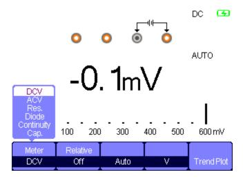
The multimeter display is 6000 counts and offers many popular test functions: including voltage, current, resistance, capacitance, diode, continuity and other test items.
