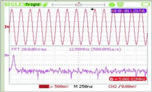
1GS/s sampling rate(single channel), 100MHz bandwidth, 2Mpts memory depth(the highest depth in handheld oscilloscope), powerful analysis and storage function, observe the details and improve efficiency
