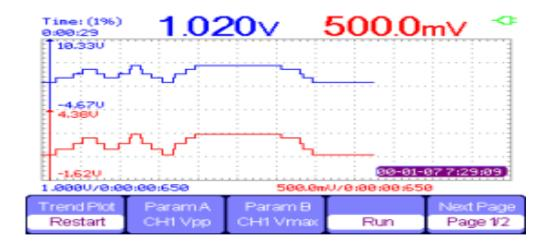
You can draw a picture to display the changes of a parameter value (measured in oscilloscope mode or multimeter mode) in a specified period of time. This is helpful to allow users to find the source of a problem quickly
