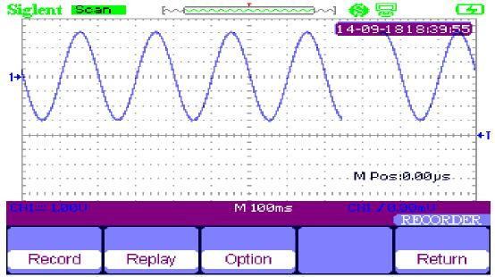
innovative recorder function, able to record waveform changes in a long time, 7M data storage space, support USB storage
