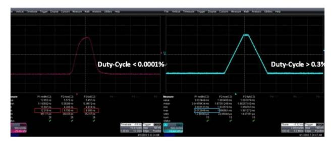
At 0.1Hz pulse, Easypulse edge can be a wide range of adjustment, the minimum edge is 6ns the maximum edge can be adjusted to 6s; but the ordinary DDS pulse edge adjustment is more restricted.
