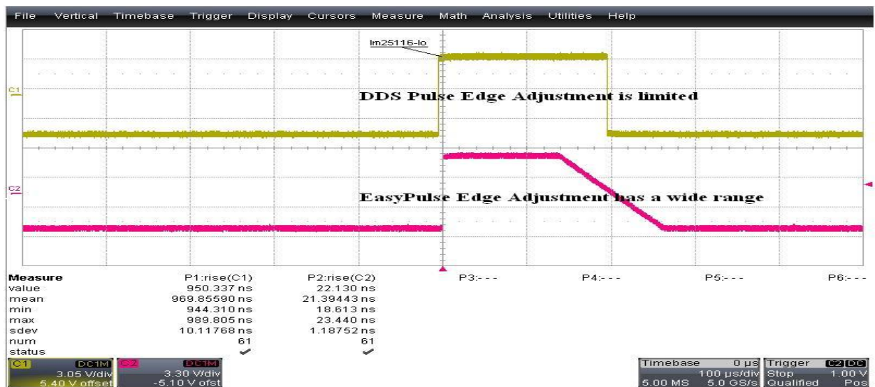
Figure 2 Comparison of edge adjusting range under 1KHz pulse signal
